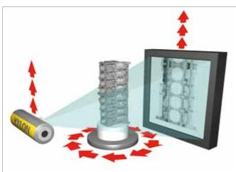
Principle of Helical CT: With stepwise rotation of the sample and stepwise vertical manipulation of the X-ray tube and the flat-panel detector all information for precise 3D volumes of long parts are obtained.
