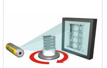
Principle of cone-beam CT: The 3D model comprises almost all information acquired by the detector during the rotation.
