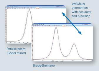
Stunning, unparalleled long-life stability and accuracy: Thanks to the unique TWIN/TWIN design, the optics return to perfect alignment within  $<\pm0.001^{\circ}$  2Theta standard deviation, a precision which cannot be achieved by manual optics changes in principle. Additionally, there cannot be any wear and possible optics damage, as the optics change is done fully automatically.
