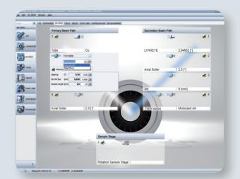
Switching between geometries is achieved using the DIFFRAC.SUITE software – the unique virtual goniometer showing all mounted components plus their status in real-time. Just mouse-click on a TWIN optics and choose the geometry – that's all!
