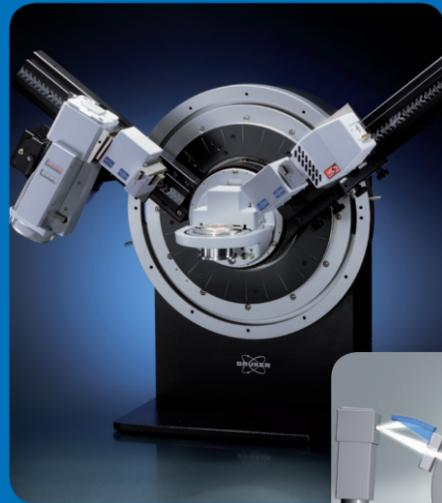
TWIN/TWIN setup for Bragg-Brentano geometry
