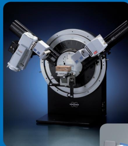
TWIN/TWIN setup for micro-diffraction
