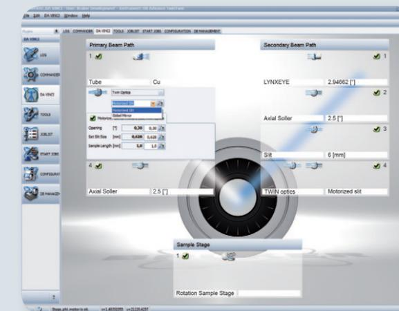
Switching between geometries is achieved using the DIFFRAC.SUITE software – the unique virtual goniometer showing all mounted components plus their status in real-time. Just mouse-click on a TWIN optics and choose the geometry – that's all!
