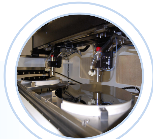
Dual Non-Immersion Imaging via Sonoscan's Waterfall™ transducer reduces contamination and false bond indications
